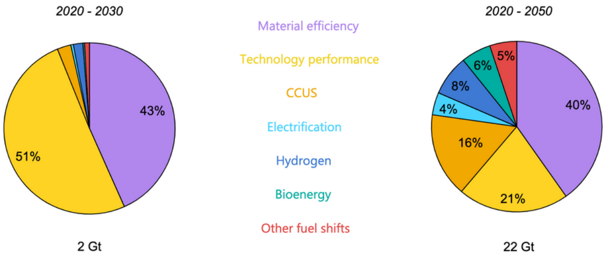
Fig. 10: Cumulative direct CO2 emission reductions in iron and steel, Sustainable Development Scenario relative to baseline
